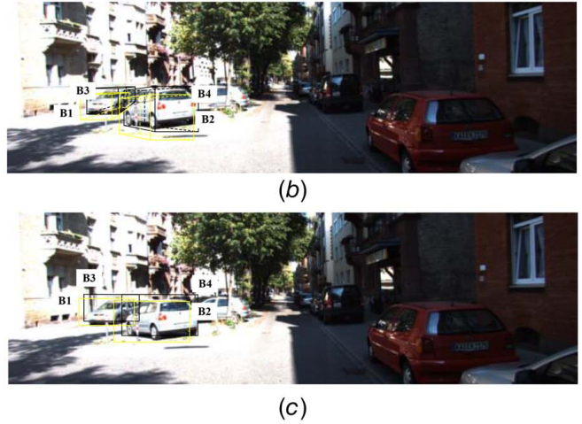
Fig. 4 Schematic diagram of 3D perspective scene: (a) schematic diagram of 3D bounding box, (b) schematic diagram of 3D multi-object tracking results, and (c) schematic diagram of 2D multi-object tracking results
